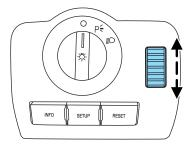
the interior lights to their minimum. The instrument panel/switch lighting remains lit.
